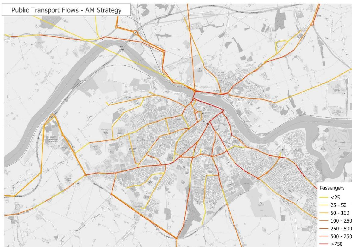
Figure 7.29: Do Strategy AM Peak Hour – PT Flow Bandwidths
