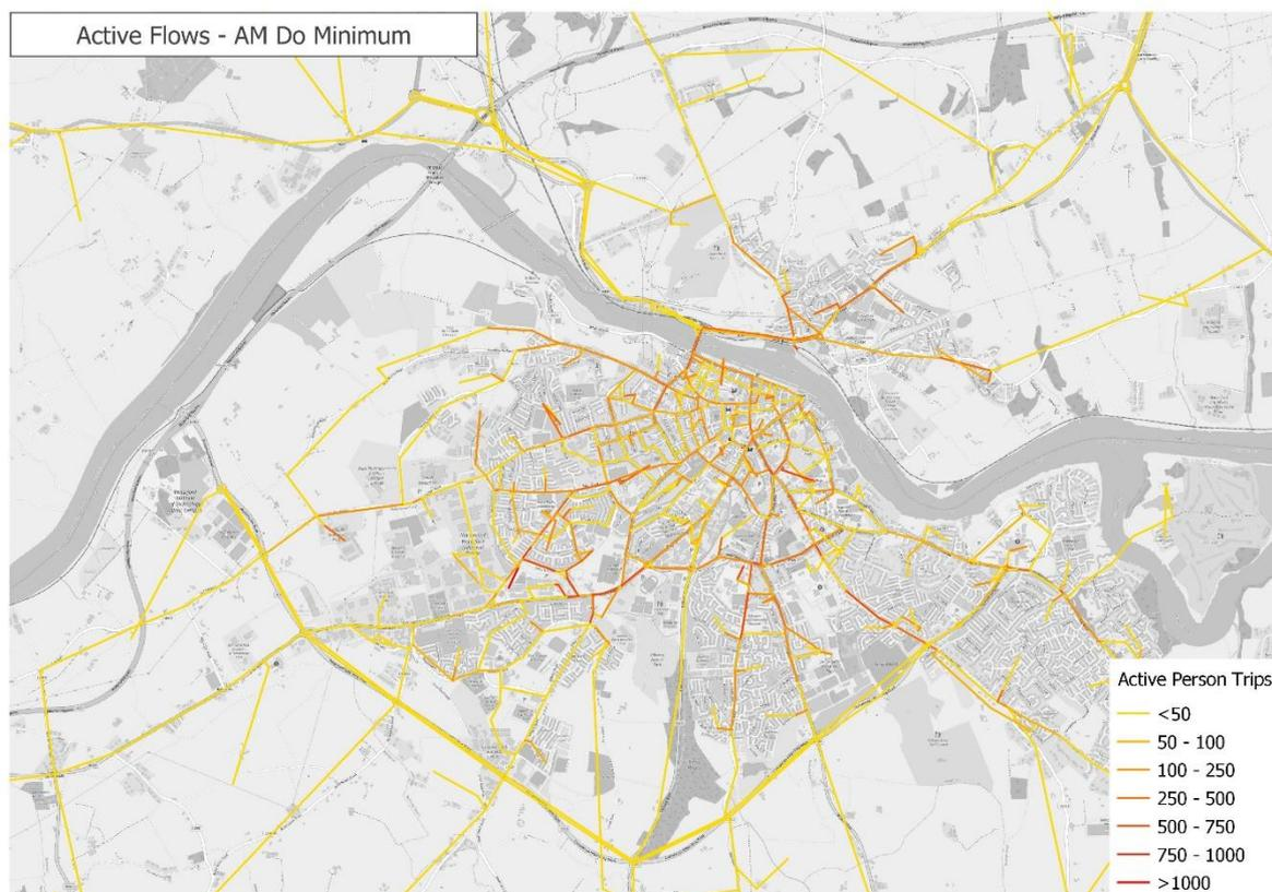
Figure 7.30: Do-Minimum AM Peak Hr Active Mode Flows
