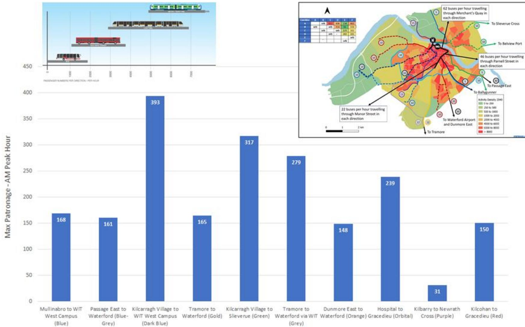
Figure 3.3 Waterford City Bus Network – Max Patronage AM Peak Hour
